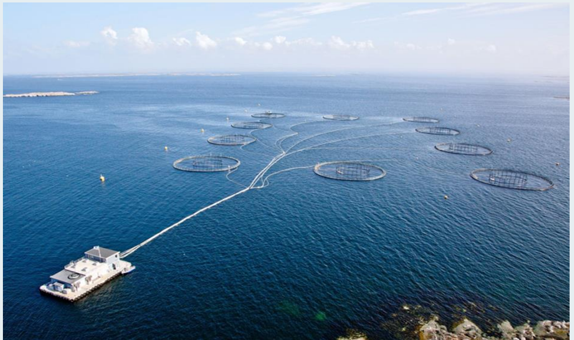
Figure 5.1: A Barge Monitors and Pumps Feed to Salmon in Net Pens at Marine Harvest Farm in Norway
